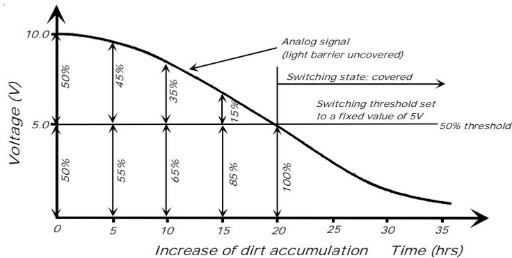
Example: The switching threshold is set to a fixed value of 5V which, in case of a 10V analog signal (without dirt accumulation and covering), leads to a change of the switching state at 50% covering of the light spot. In case of increasing dirt accumulation the analog signal decreases, while the switching threshold remains constant. This means that the light spot no longer has to be covered by 50% in order to cause switching of the light barrier.
