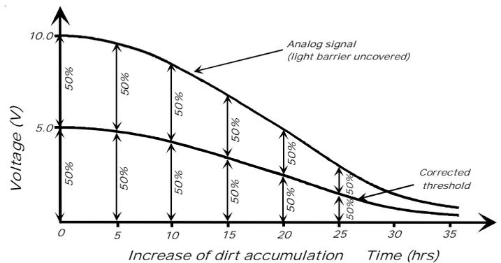
Example: In clean condition the laser light barrier of series F-LAS indicates a value of 10V at the analog output, the switching threshold adjusts itself to 50% of the analog signal, i.e. the switching state changes at 50% covering of the light spot. In case of increasing dirt accumulation the value of the analog signal decreases, but the 50% distance to the switching threshold is maintained.
